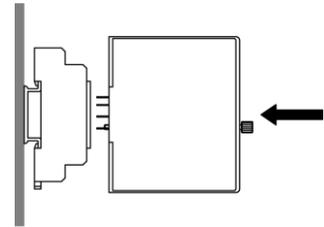
3) How to disconnect the main unit from the socket
