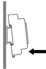
2) How to secure the main unit to the socket
