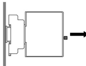
4) How to disconnect the socket from the socket
